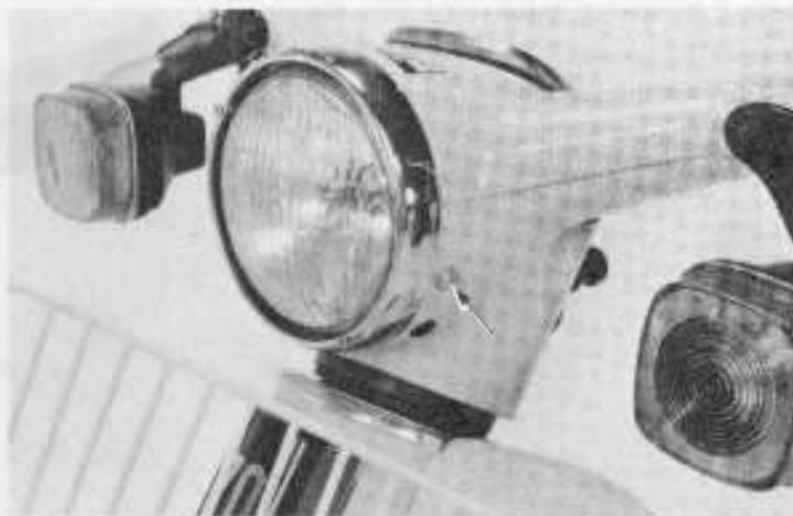
Remove the right handlebar switch mounting screws.
