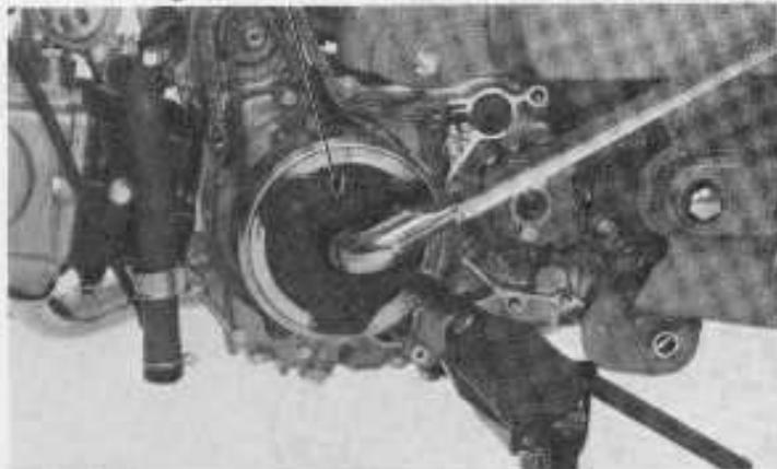
Install the stator on the left crankcase cover with the screws.
