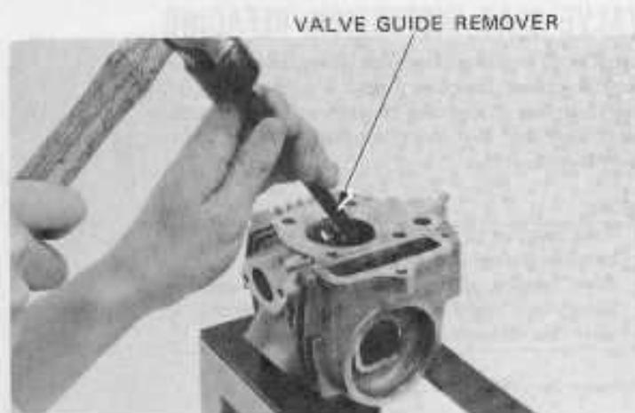
Install a new oversize valve guide from the top of the head.
