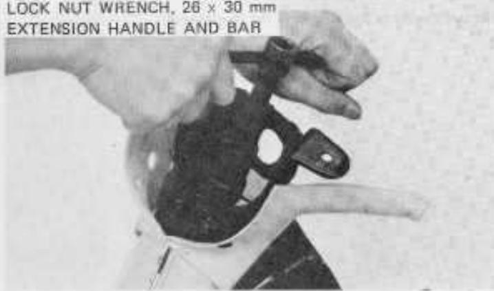
Remove the bearing adjusting nut.
