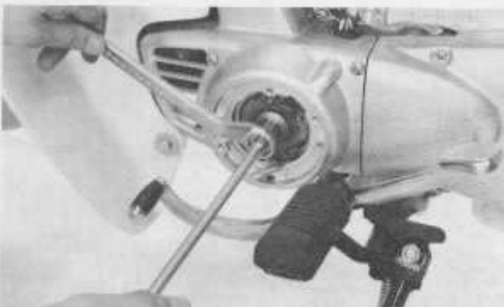
Install the advancer, aligning the slot with the flywheel pin.
