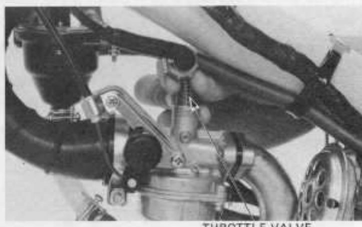
Compress the throttle valve spring and remove the throttle cable from the throttle valve groove.
