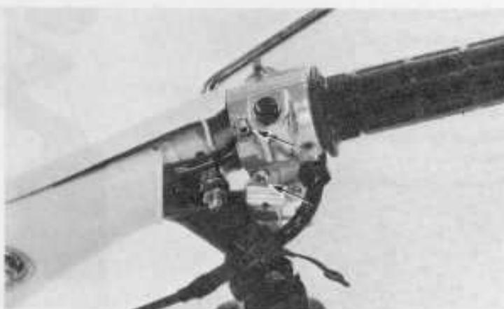
Disconnect the throttle cable end and remove the throttle grip.
