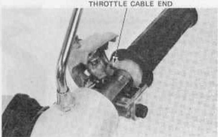
Remove the left handlebar switch mounting screws.
