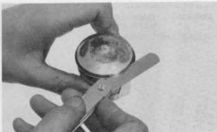
Insert each piston ring into the cylinder, and measure the end gap.
