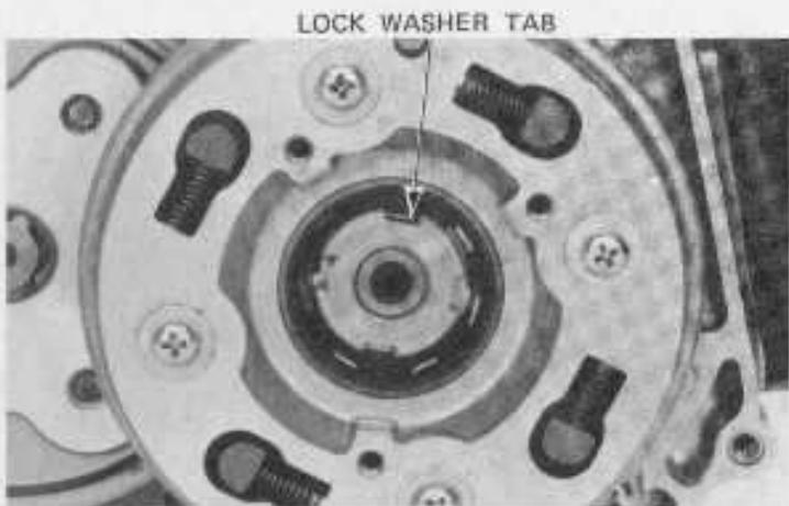
Remove the lock nut, washer and lock washer.
